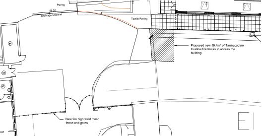
Proposed Weld Mesh Fenching and Gates
